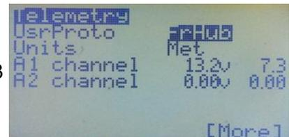
The number in the right hand column represents the final Telemetry read-out (in the picture, 7.3V). If it does not agree exactly with the actual value measured with a voltmeter, the range value can be adjusted slightly. The usual cause of inaccuracies in the reading is the tolerance of the resistors used in the voltage divider.
