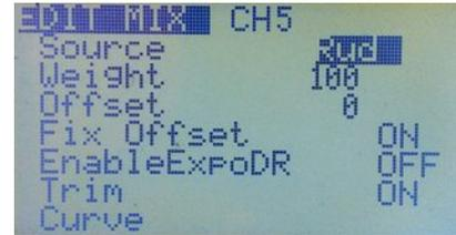
It's important to understand that in the Er9x kind of programming, the only way anything can be controlled is through an explicit mix. In many other radios, most of the mixes are built-in but hidden; here they are fully visible and editable, giving the radio enormous flexibility and power, but requiring that, except in the case of the default mixes for a new model, you create the mixes yourself.
