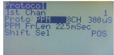
**Number of Channels:** Can be set from 4 to 16 in increments of 2. This is important when using the TX with some flight simulator dongles that can't accept more than 4 or 6 channels.
