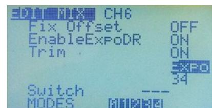
The pictures above show each of these three options. Use the [LEFT] and [RIGHT] keys to select the one you want to apply to the mix. Pressing the [DOWN] key highlights the value under the words “Curve”, “Diff” or “Expo”. The [LEFT] and [RIGHT] keys adjust the values. The range of possible values for Expo and Diff is 0 to +/- 100.
