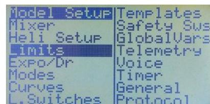
Select a menu using the [UP]/[DOWN] and [LEFT]/[RIGHT] keys, then press [MENU] to open it. The list of menus begins with Mixer, the focal point of programming.
