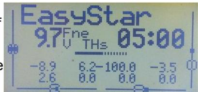
**Warning:** It's easy to give a short [RIGHT/LEFT] press inadvertently and display channels not being used on your transmitter.
