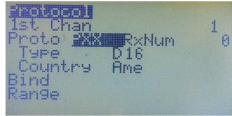
**RxNum** - Receiver match. This gives the receiver a number (0...124) to prevent you from flying with the wrong model selected in the radio.
