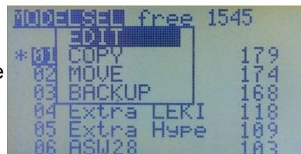
Press short [RIGHT] or [LEFT] to directly enter the *Model Setup* index page for the chosen model. Don't be surprised if you see an ALERT screen telling you that THROTTLE needs to be moved to idle, and/or the switches must be in their default position. For your safety, the throttle stick and switch positions are checked every time you change models, not just when the transmitter is turned on. This important safety feature can be turned off if desired, but doing so is not recommended.
