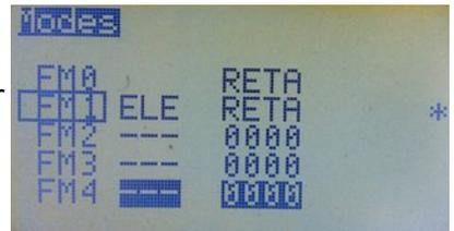
Flight Modes can also be used to determine which mixes are turned on for each mode. The Edit Mix menu (see below) allows the mode(s) in which a mix is active to be selected; by default a mix is active in all Flight Modes.
