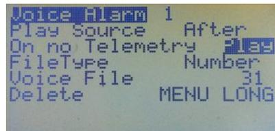
The voice file number 0031 (flight battery low) will play once (Rate is set to “ON”), if the source (A1=) drops below 7.2V (v<val = A1<7.2V), followed (AFTER) by the voltage report (Play Source). The radio will vibrate at the same time (Haptic1).
