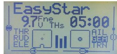
In the upper half of the screen, the transmitter voltage is displayed in large print, along with the trim increment type, here 'Fne' (see page 68). The current value of the Timer is also shown in large print, along with the trigger used to activate it, here 'THs' (see page 64). In addition, the active Flight Mode will be displayed if it is other than the default FM0, replacing the trim increment type on the screen, as shown in the picture at right.
