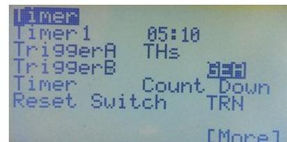
To set the time in steps of one minute highlight the field and press and hold the [MENU] key while setting the time.
