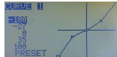
You will see 5 or 9 editable points with the values initially set at zero. Scroll through the points with [UP/DOWN]. Change the value with [LEFT/RIGHT].
